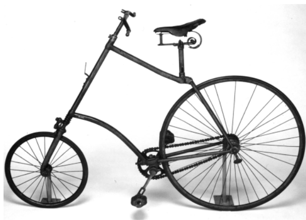
図15 Humber Safety Bicycle(1885) [回転ペダル式後輪チェーン駆動型自転車] [出典] David V. Herlihy (2004), Bicycle , p.237
